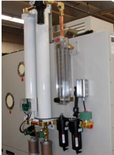
Fresh Air Exchange System - Aids in removing all gases from inside the chamber prior to opening the door
