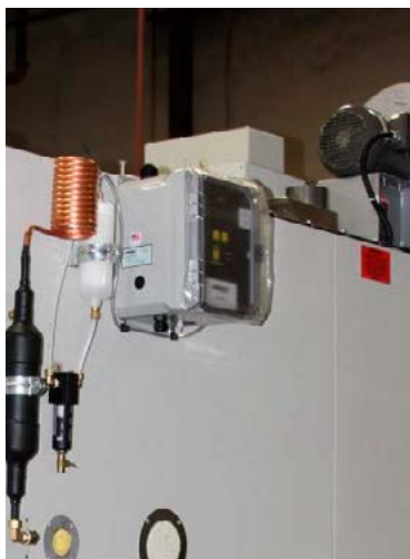
Gas Monitors - O 2 , H 2 , CO, etc - Can be interlocked to controller to shut down chambers
