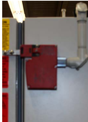
Safety Door Interlock - Prevents entry either during tests or after an event
