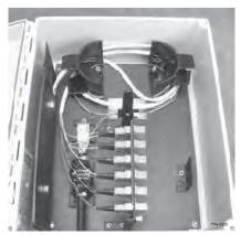
Step 1: Place completed tray(s) into the holder and secure with the hook-and-loop strap (make sure the buffer tube(s) and pigtail(s) are routed around the radius control guides as shown).
