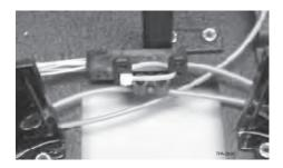
**NOTE:** For both applications, route the connectorized fan-out tubing around the radius control guides and plug connectors into the appropriate connector panel.
