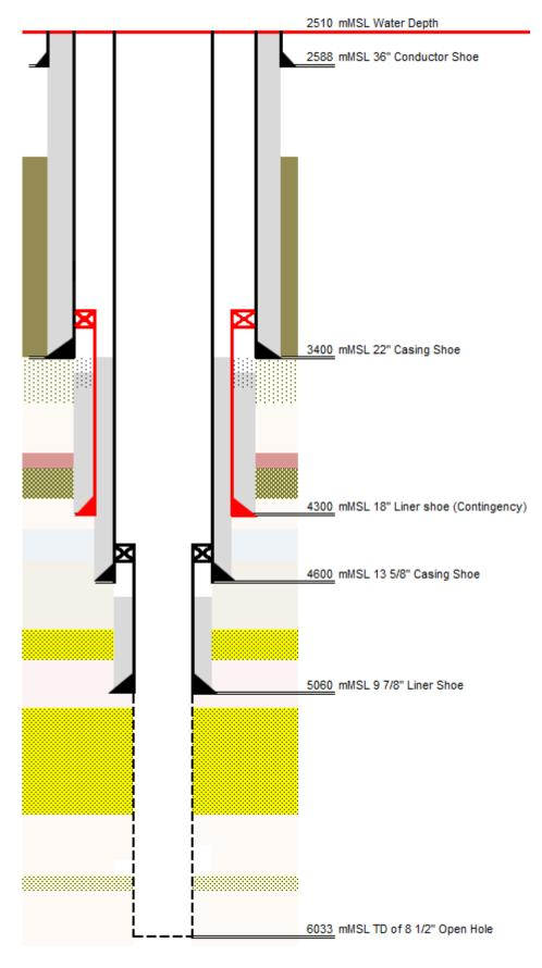
*Figure 3-9* Schematic outline of the Mronge-1 exploration well (with contingency string). (Source: Statoil)
