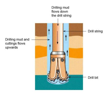
*Figure 3-7* Schematic illustration of circulation of drilling mud and cuttings in the drill bit (Source: COWI)
