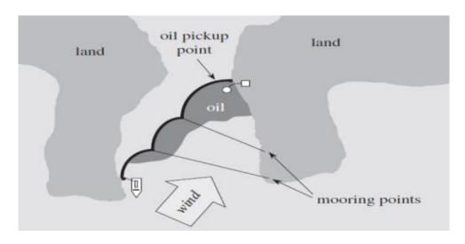
*Figure 8-2* Sketch of the way shoreline protection booms are functioning. (Source: Statoil)
