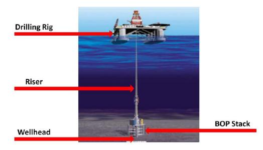
Figure 3-8. Schematic view (not to scale) of a riser on a semi-submersible rig, similar to that used on a drill ship (Source: COWI)
