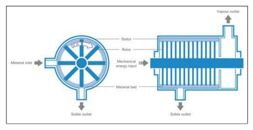
Figure 8-4 Sketch of a TCC unit (Source: Thermtech A/S)
