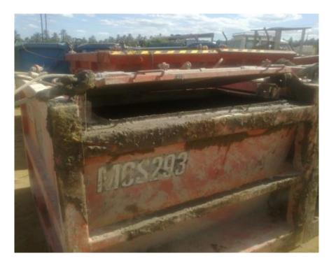
Figure 7-10 Skip container for transport of cuttings (Source: COWI).
