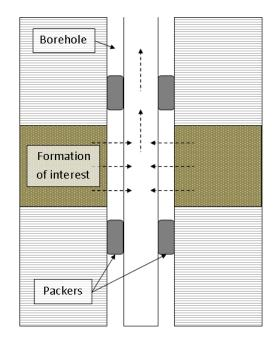
Figure 3-13. Schematic view of Drill stem testing.(Source:COWI).
