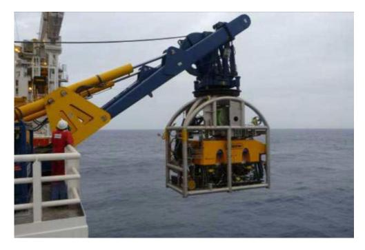
Figure 3-6 Remotely Operated Vehicle being launched (Source: SERPENT project)
