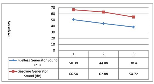
Figure 2 : Noise level variation between fuel less Generating set and Gasoline type
