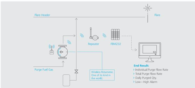
network, while higher purge quantities could lead to excess burning of fuel gas and emissions into the atmosphere. Less purging would allow for the ingress of air and moisture that could create problems like pipe corrosion flame out of flare. Higher purge quantities would burn the expensive fuel gas and impact the environmental Key Performance Indicators.
