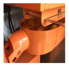
Figure 3. Removing the juicing parts during routine maintenance. (Photo Source: Saudi Aramco)
