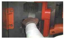
Figure 2: The feeder from the orange hopper to the juicer. (Photo Source: Saudi Aramco)
