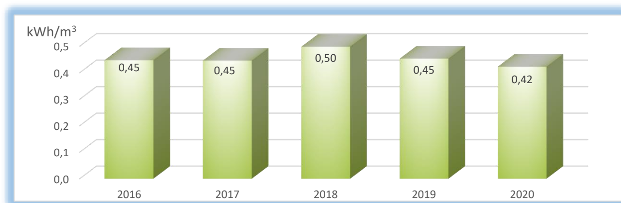
Chart 8: Electricity consumption per unit produced at the wastewater treatment plant in 2016-2020, kWh/m 3
