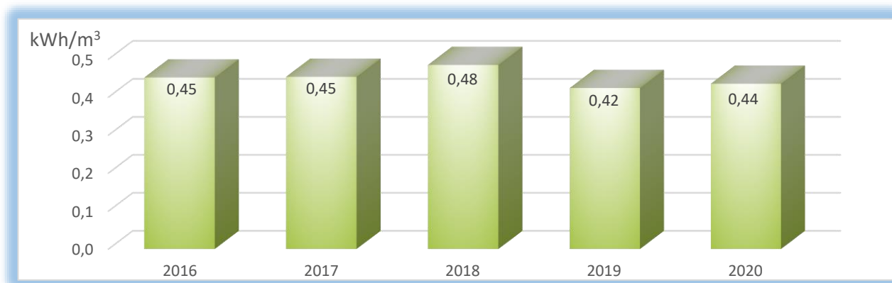
Chart 7: Electricity consumption per unit produced at the water treatment plant in 2016-2020, kWh/m 3
