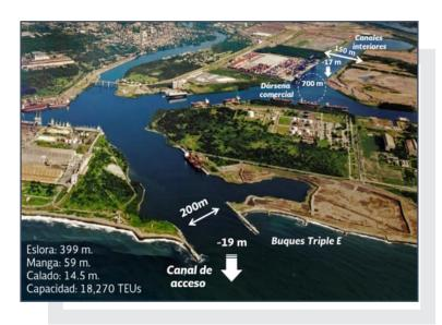
Lazaro Cardenas' Port has 18 berths with a total length of 6,358 m, making up 15 port terminals, the access channel has a length m 1.740 internal channels have a total length of 7,818 m. It has an anchorage of 1330.32 hectares.
