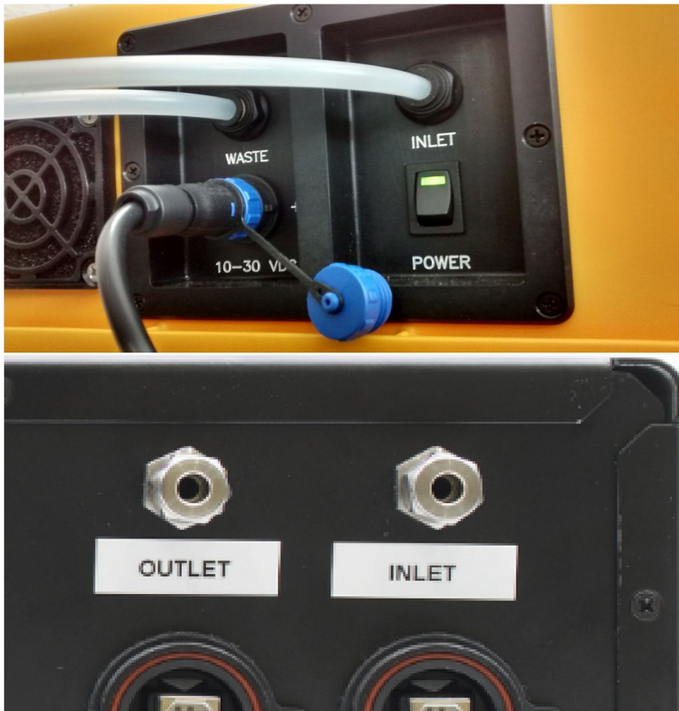
Figure 5 Top: Inlet and Waste push-connect ports on the UGGA. Bottom: Inlet and Outlet ports on the eosMX.
