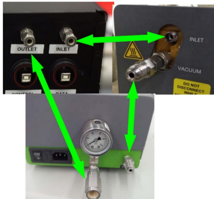
Figure 1 Gas tubing connections between the analyzer, eosMX and external pump.
