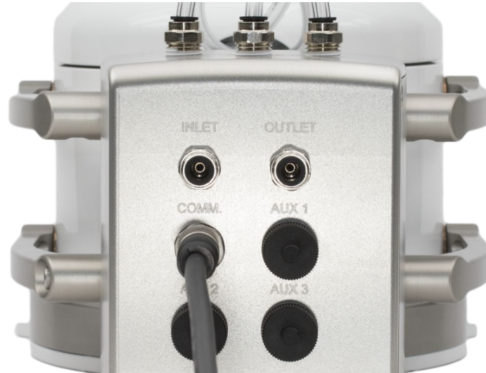
Figure 7 Power/Data Cable connected to the eosAC
