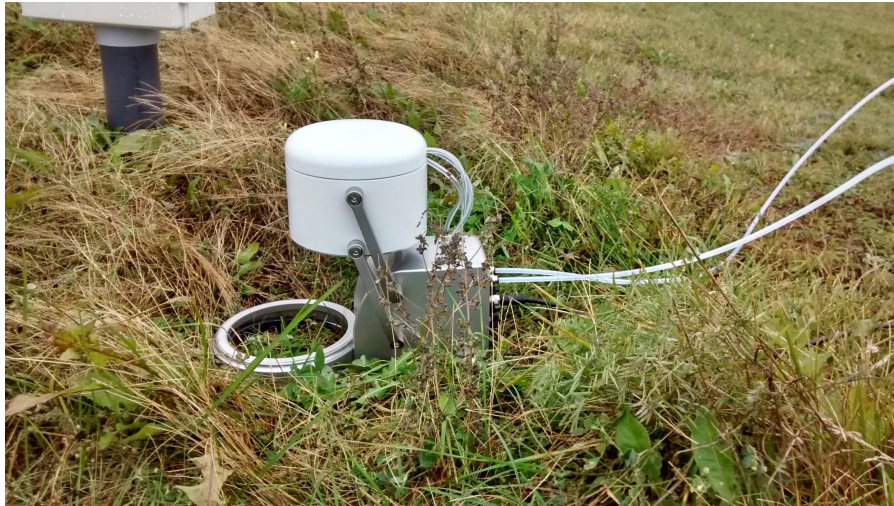
Figure 9 An eosAC deployed in the field using a simple PVC collar.
