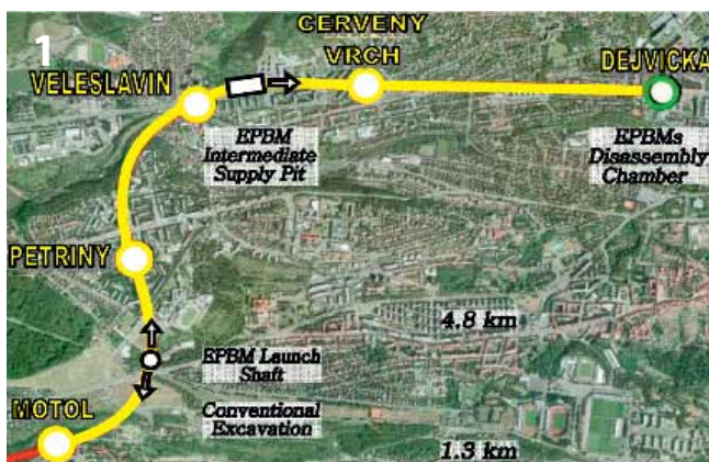
Metro V.A. will add to operation 4 new stations and 6.1 km of tunnels to the existing Prague subway
