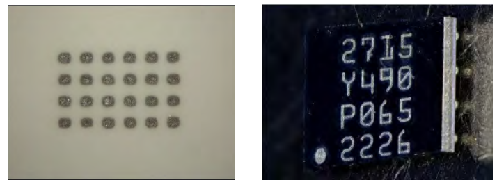
Figure 31: (Left) Solder stencil pattern squeegeed onto ceramic substrate. (Right) EPC2715 after reflow onto substrate.
