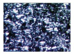
Figure 3 Cross Section of Paraffin Wax Modified With 1% *Epolene* Polymer
