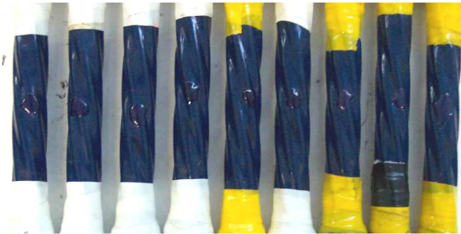
Test result of 3,000 hour salt spray test with epoxy patch kit repair on an artificial crack
