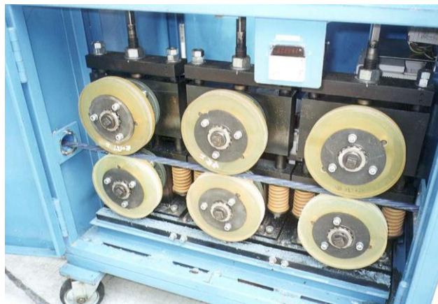
Pushing machine specially designed for ECS
