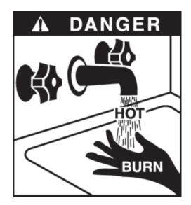
**WARNING:** Studies show that dangerous bacteria can form in domestic water distributions systems if a minimum water temperature is not maintained. For example, legionella pneumophila, can form in hot water maintained at 115°F (46°C) or lower. We recommend a domestic water temperature not lower than 122°F (50°C) at faucets and a tank temperature not lower than 140°F (60°C) to limit the potential for legionella pneumophila growth. Contact your local health authority for more information.
