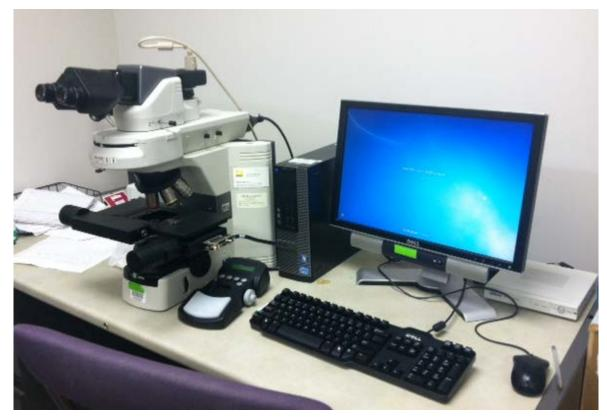
Motorized stage with image stitching software
