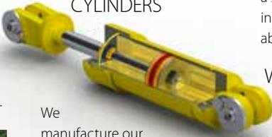
We manufacture our own industrial cylinders with induction hardened chrome shafting, urethane seals and wear bands to eliminate scarring and oil contamination. Shorter strokes translate into rapid movements and more wear, so we developed our center cylinder with a longer, smoother stroke to increase life expectancy and reduce wear and tear.
