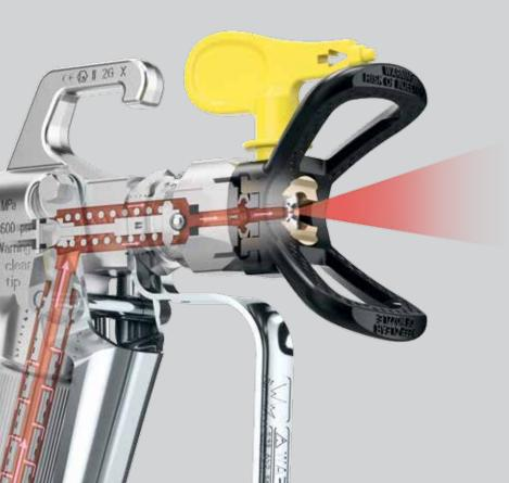
Unlike the case of air atomisation, airless atomisation technology atomises the material using the pressure of the material alone, i.e. without the use of any air.
