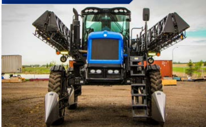
2013 New Holland SP275R 120/70' 1200G Poly, 380/90R46 Tires, Duals, Capstan Rate Sys, Crop Dividers, Factory Autosteer...
