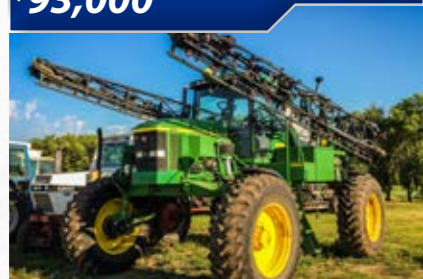
2001 John Deere 4710 90' 800g SS Tank, JD 2600 w/Globe and Autosteer, 5 Sec, 380/90R46 & 520/85R38, Norac Height Control...
