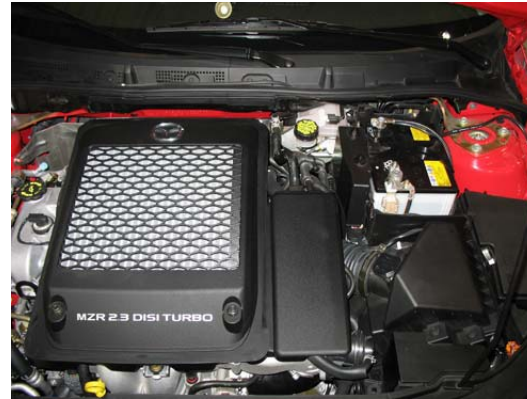
b) Remove the two bolts securing the plastic intercooler shroud. Remove the shroud.
