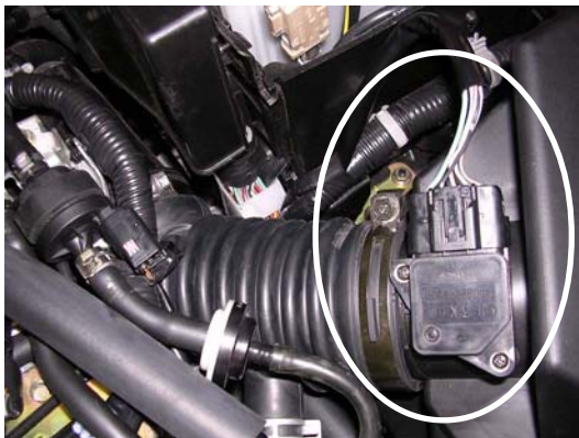
c) Unplug and remove the mass air flow sensor (MAF) wiring harness.
