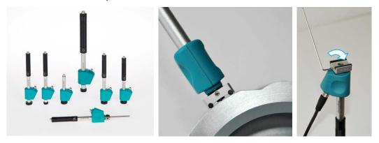
Figure 12: Overview of Equotip 550 Leeb Impact Devices and usage of support rings
