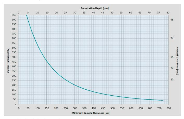
Figure 6: Portable Rockwell conversion curve
