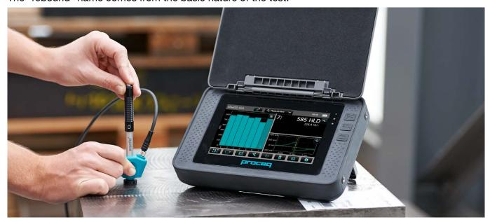
Figure 5: Eqoutip 550 Leeb hardness testing instrument
