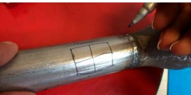
Figure 25: Preparation of test sample and marking of the test area
