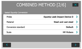
Figure 23: Screenshot of settings for the Leeb measurements
