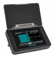
The new Equotip 550 is an all-in-one solution combining the Leeb, Portable Rockwell and UCI methods and is compatible with upcoming developments, such as other measuring principles and new types of probes etc. The new-generation display unit with touchscreen leverages the high measuring accuracy with an unmatched user experience leading to increased measurement efficiency.
