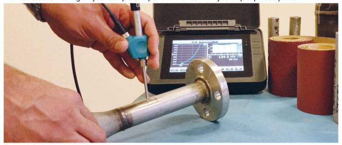
Figure 26: Performing Leeb measurements on test sample
