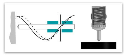
The UCI method uses the same pyramid-shaped diamond as a conventional Vickers hardness tester. Unlike Vickers testing, no optical evaluation of the indentation is required, enabling fast and portable measurements. The UCI method excites a rod into an ultrasonic oscillation. The test load is applied by a spring and typically ranges from 1 to 5 kg of force (HV1 – HV5). As the diamond is forced into the material, the
