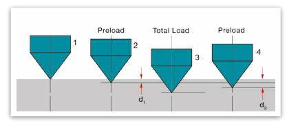
The Portable Rockwell metal hardness tester is based, as its name suggests, on the static Rockwell measuring principle where the penetration depths under a defined preload are measured before and after application of a large force.
