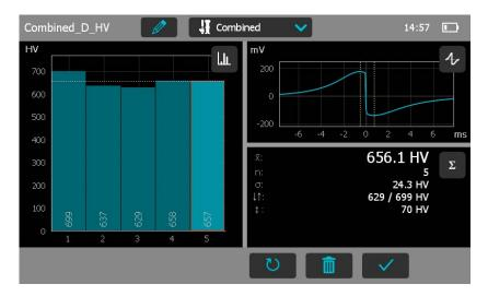
Figure 27: Equotip 550 after five performed measurements
