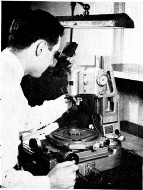
Checking a geneva wheel with a toolmaker's microscope
