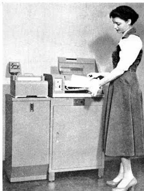
Letter to be scanned is placed between cylinder and transparent plastic wrapper of new model Telefax transmitter. Recorder is at left
