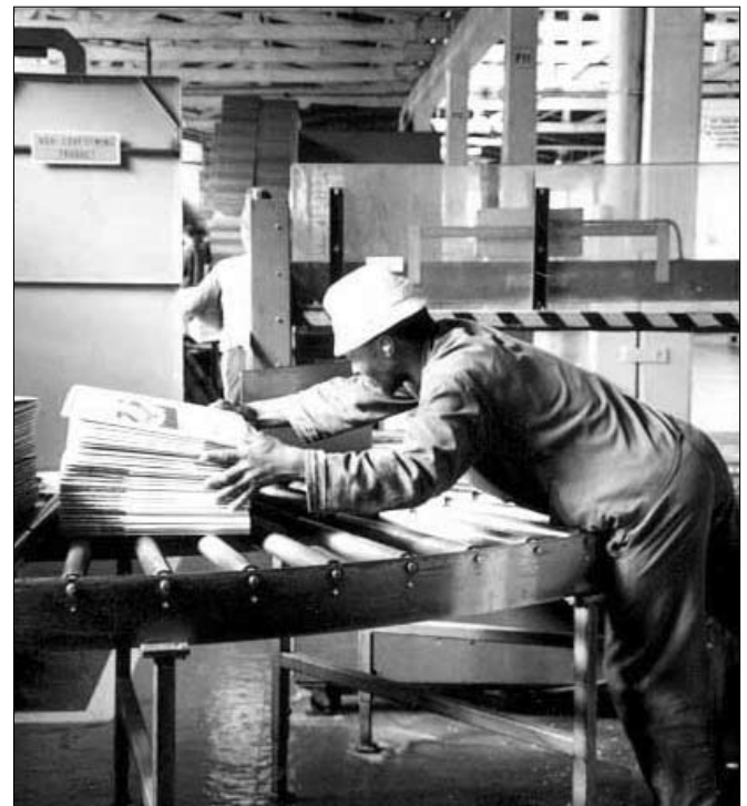
Figure 7 Excessive and unnecessary reaching.
