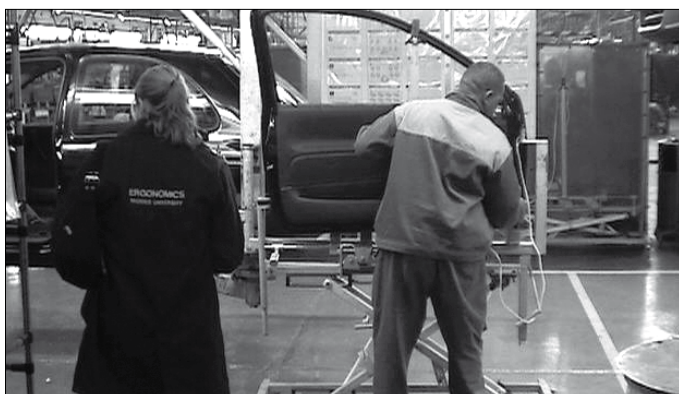
Figure 18 Moveable stand to hold car door reduces strain and the risk of injury.
