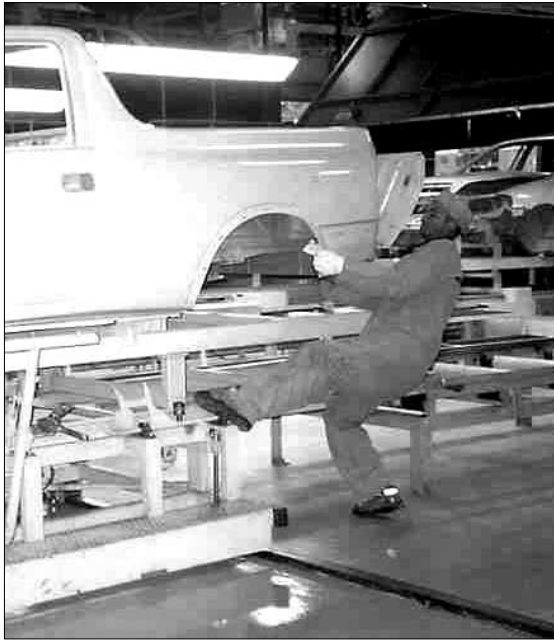
Figure 10 Unbalanced work posture and use of excessive force such as in this task can be the result of local conditions. Local solutions may be relatively easy once the problem is acknowledged.
