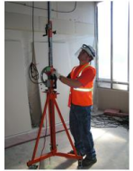
Overhead drill press developed as a CPWR research project. Photo courtesy of Dr. David Rempel.
