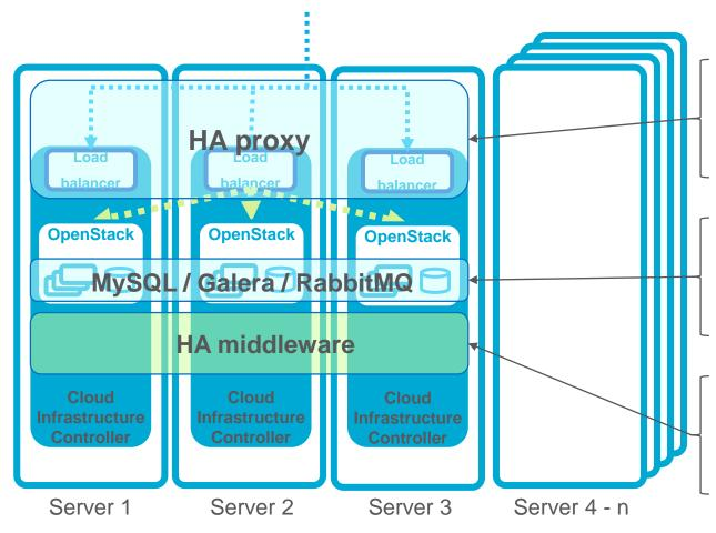
Load balancing functions using **HA Proxy** nodes ensures robust and scalable access to the OpenStack functions.
