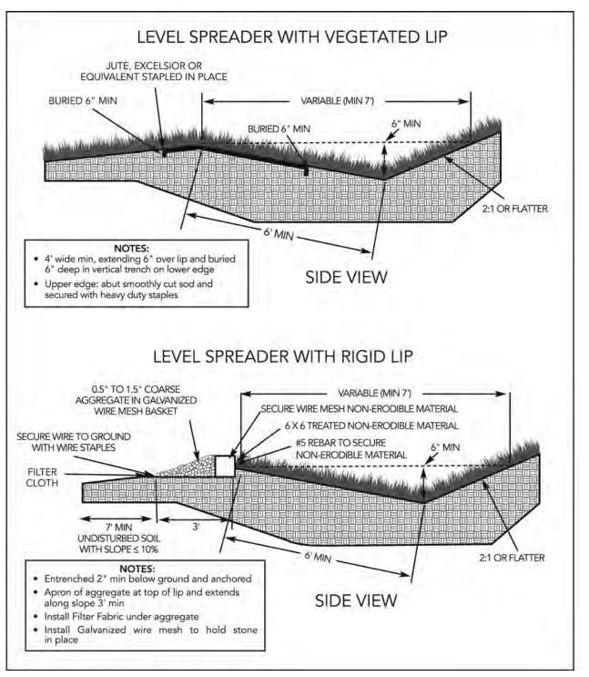
Figure 9-19 Level Spreader Cross-Section
