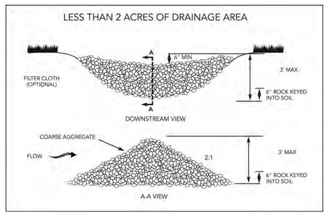
Figure 9-15 Rock Check Dam – Less Than 2 Ac.
