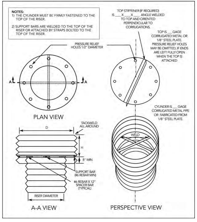
Figure 9-36 Anti-Vortex Device Design
