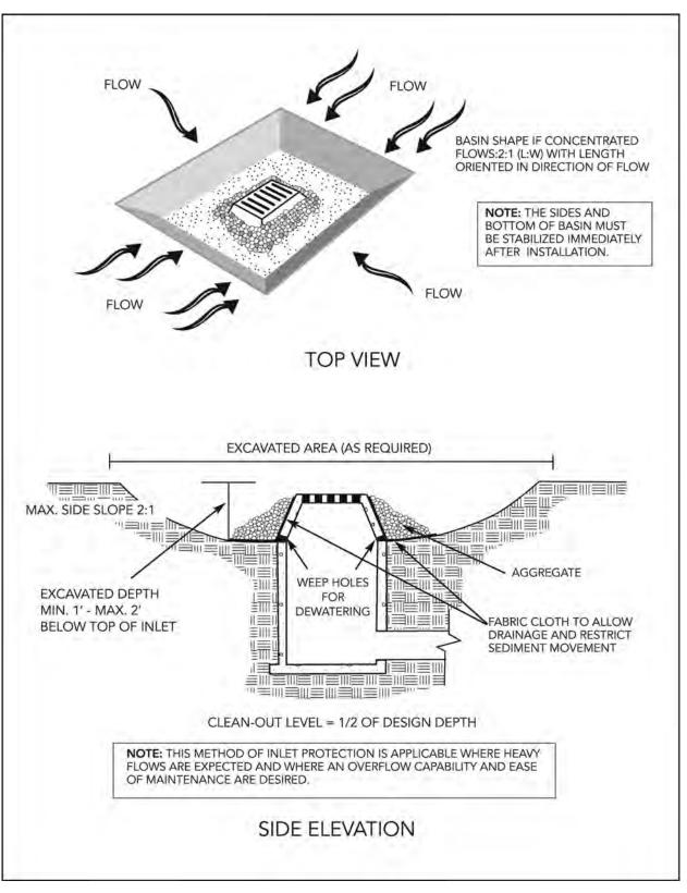
Figure 9-6 Excavation Drop Inlet Sediment Trap
