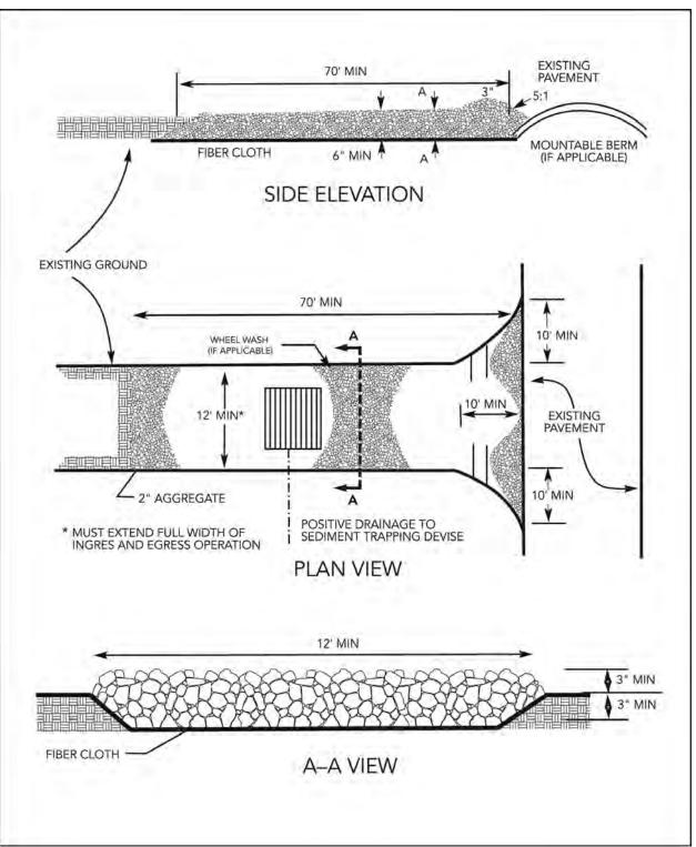
Figure 9-3 Aggregate Construction Entrance
