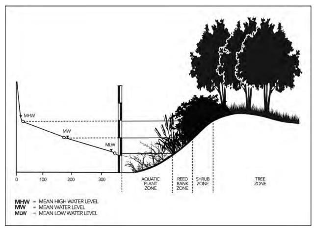
Figure 9-41 Typical Annual Curve of Water Levels Correlated with Typical Vegetative Zones.
