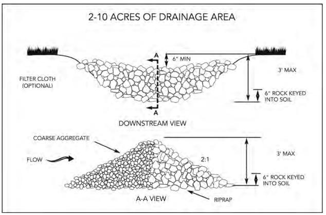
Figure 9-16 Rock Check Dam – 2-10 Ac.
