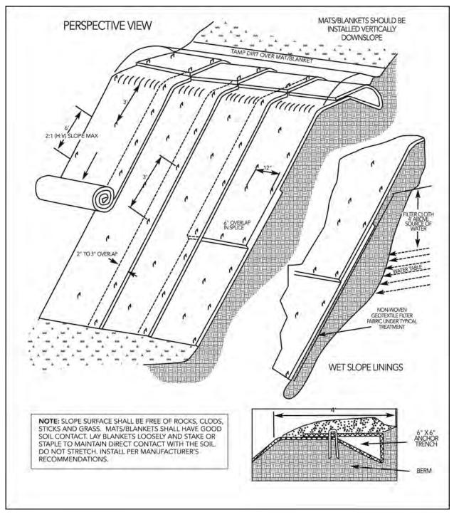
Figure 9-51 Typical Treatment – 2 Soil Stabilization - Matting Installation
