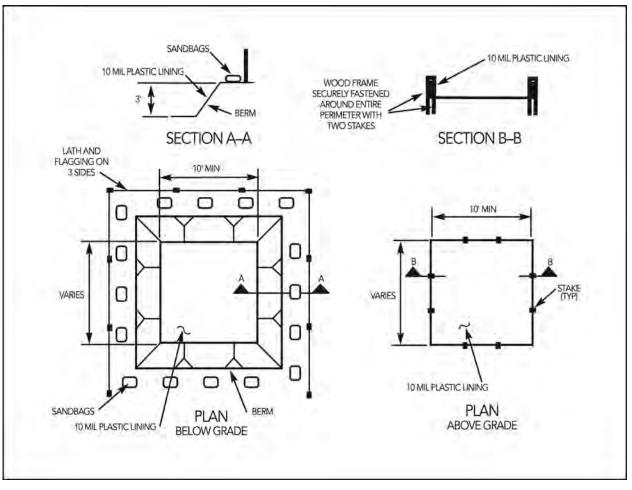
Figure 9-62 Installation of Below Grade Washout Facility
