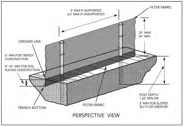
Figure 9-4 Silt Fence Installation
