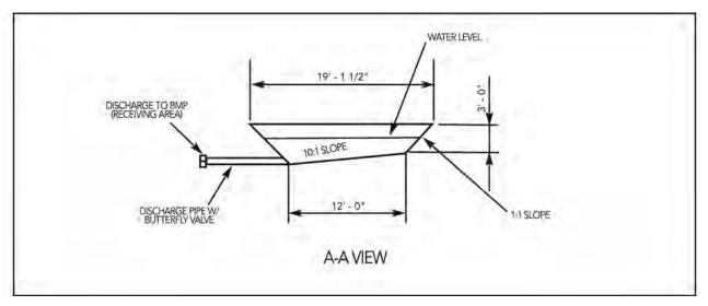
Figure 9-55 Wheel Wash Section (Section A-A)
