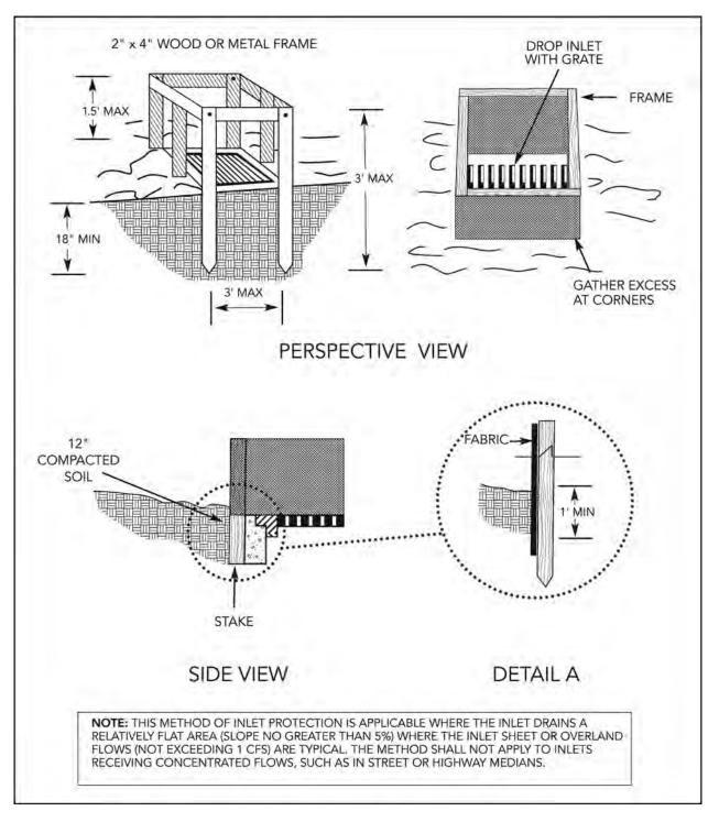
**Figure 9-7 Silt Fence Drop Inlet Protection**
