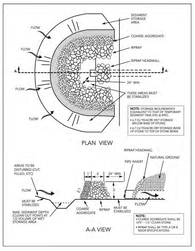
Figure 9-12 Culvert Inlet Sediment Trap
