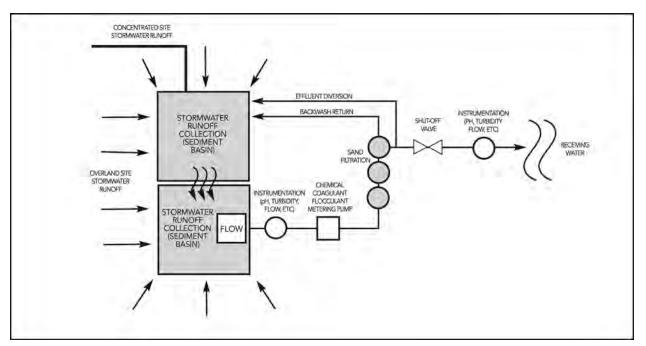
Figure 9-59 Typical Flow-Through Treatment Process
