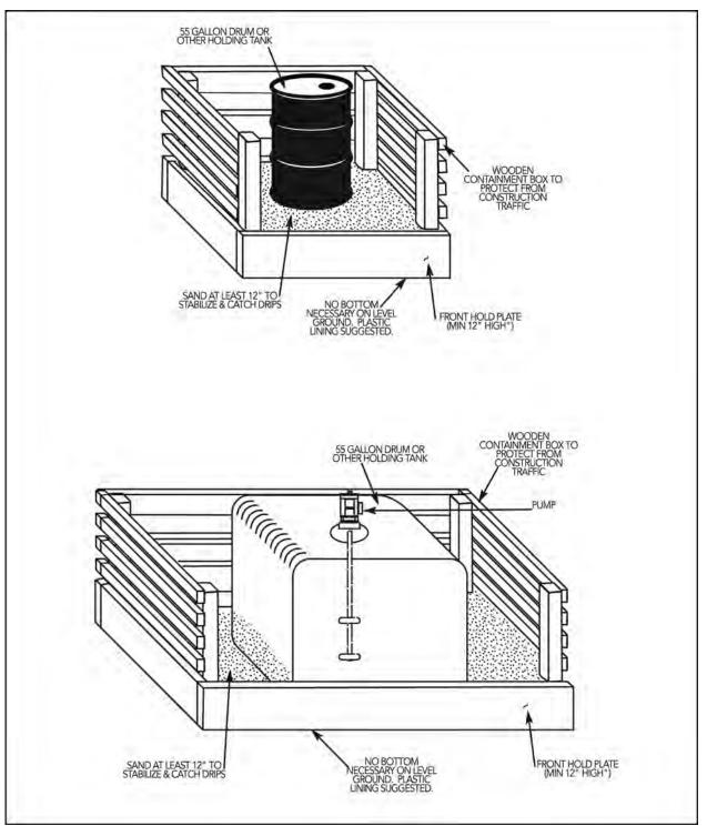
Figure 9-60 Spill Control Structures
