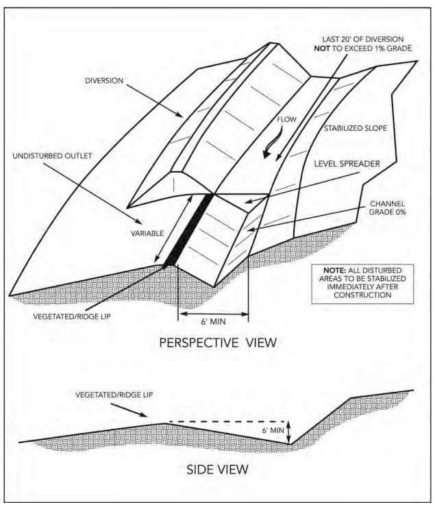
Figure 9-18 Level Spreader Perspective View
