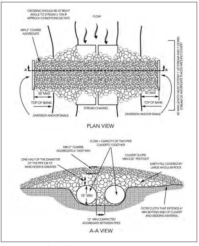
Figure 9-22 Temporary Culvert Crossing
