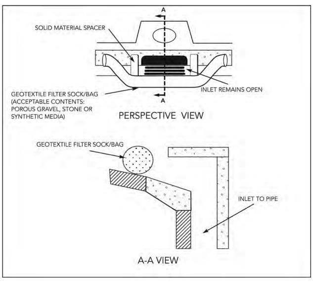
Figure 9-10 Curb Inlet Protection With Filter Sock
