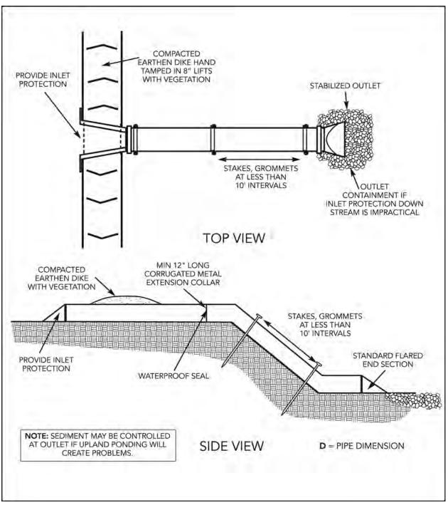
Figure 9-20 Temporary Slope Drain
