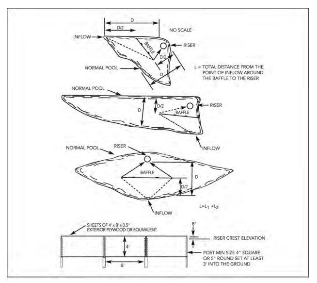
Figure 9-29 Baffle Locations In Sediment Basin
