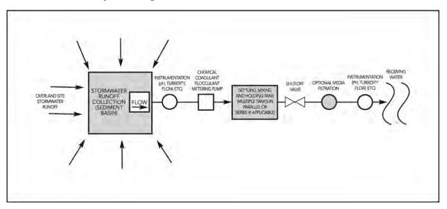
Figure 9-58 Typical Batch Treatment Process
