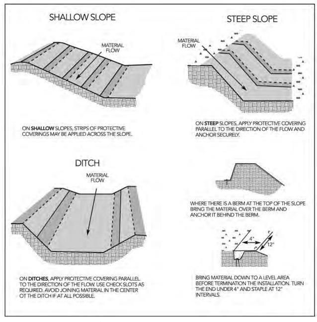
Figure 9-47 Typical Orientation of Treatment – 1 (Soil Stabilization Blanket)
