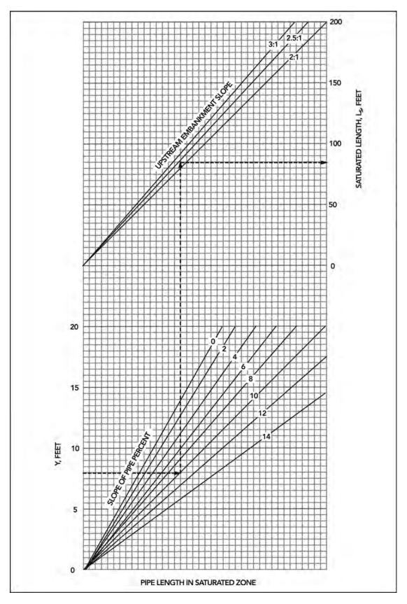
Figure 9-37 Pipe Length In Saturated Zone
