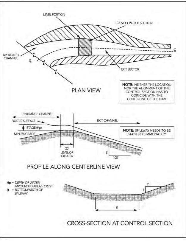
Figure 9-35 Excavated Earth Spillways
