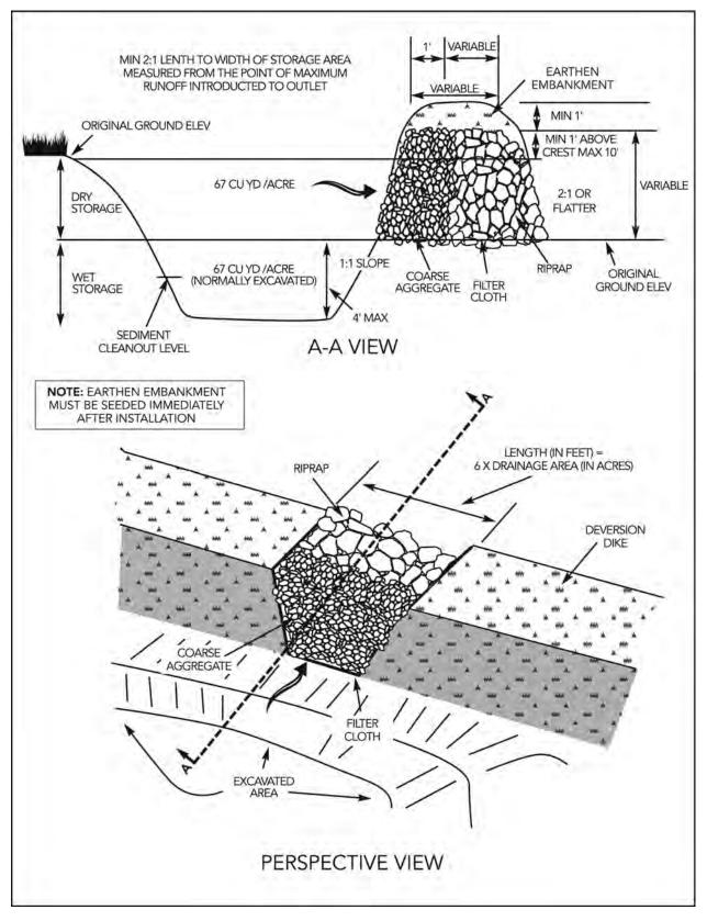
Figure 9-26 Typical Temporary Sediment Trap
