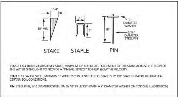
Figure 9-48 Typical Treatment – 1 Installation Criteria (Soil Stabilization Blanket)
