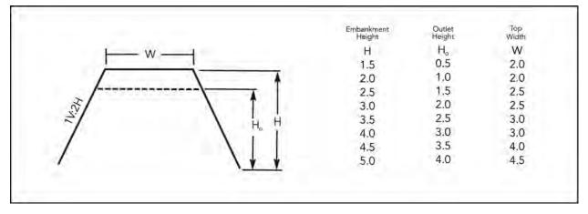
Figure 9-27 Minimum Top Width (W) Required for Sediment Trap Embankments According to Height of Embankment (Feet)
