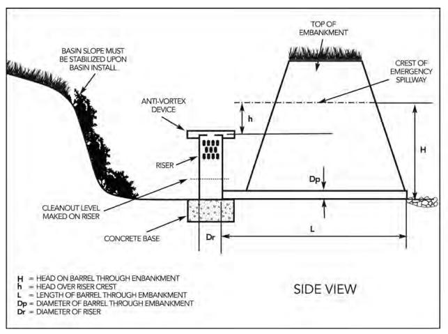
Figure 9-31 Principal Spillway Design
