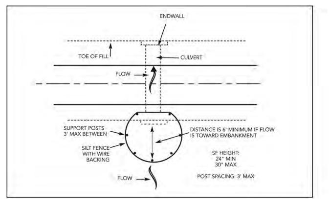
Figure 9-11 Silt Fence Culvert Inlet Protection
