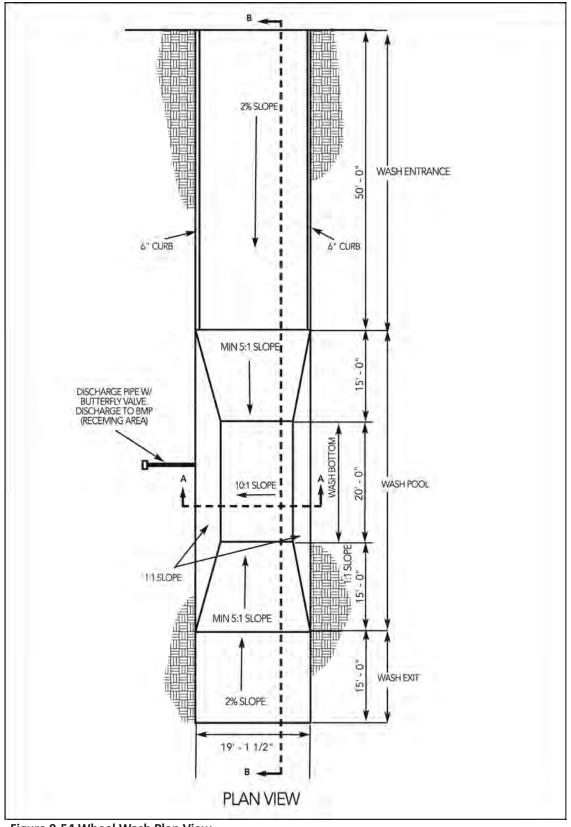
Figure 9-54 Wheel Wash Plan View
