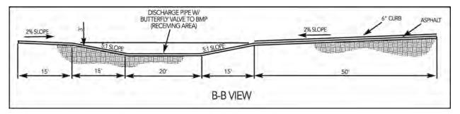
Figure 9-56 Wheel Wash Elevation View (Section B-B)
