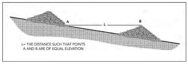
Figure 9-17 Spacing Between Check Dams
