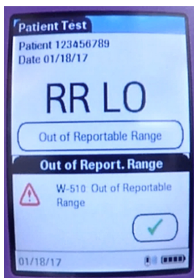
Figure 1. Accu-Chek Inform II glucometer displays the blood glucose with an abbreviation, RR LO (out of reportable range; low limit) and an alarm code, W-510 Out of Reportable Range, below the abbreviation. The "510" in the alarm code has been mistaken as the blood glucose value, leading to the incorrect administration of insulin (source of photo: VHA 8 ).
