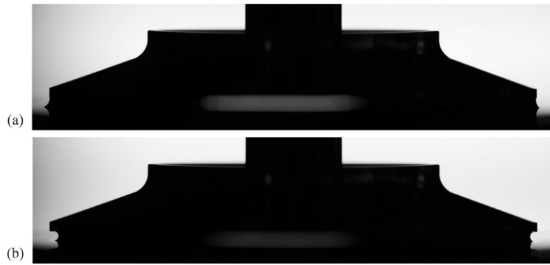
Figure 1. Rheometer setup for a parallel plate head, (a) properly filled sample, (b) under-filled sample.
