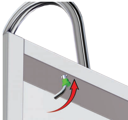
Fig. 9: Secure spout with bushing
