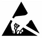
The ESD Susceptibility Symbol (also called Sensitivity or Warning Symbol) identifies items that can be damaged by ESD and should be unpackaged and handled while grounded at an ESD protected workstation.
