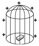
To complete the enclosure, make sure to place lids on boxes or containers, and close shielding bags. Packaging with holes, tears, or gaps should not be used as the contents may be able to extend outside the enclosure and lose
