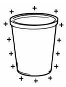
Insulators like this plastic cup will hold the charge and cannot be grounded and "conduct" the charge away.
