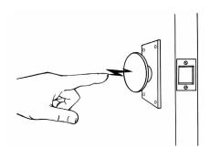
The occasional zap felt when sliding out of an automobile and touching the door handle In a normal environment like your home, there are innumerable ESD events occurring, most of which you do not see or feel. It typically takes a discharge greater than 2,000 or 3,000 volts for a person to feel the "zap." It requires a much larger ESD event to arc and
