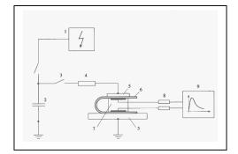
Fig. 2. Structure of the test build up [3]
