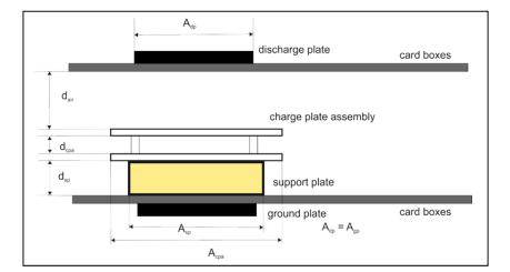
Fig 3. Shielding measurement assembly in a card box
