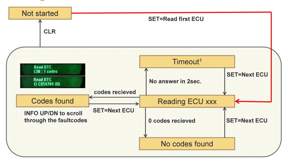
1) Timeout will occur if the vehicle is not equipped with the ECU or if the ECU is broken or missing power supply/CAN-bus
