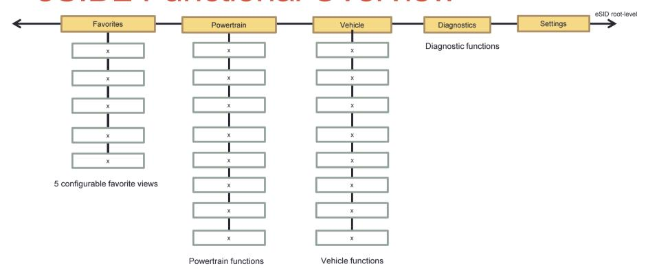
Only relevant views are displayed to the driver, for instance: No XWD data on FWD vehicle and no Ethanol view on Diesel vehicles.
