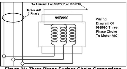
Figure 21: Three Phase Surface Choke Connections
