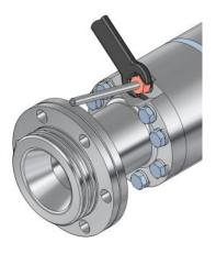
Tighten nut to 25 ft•lbs. Or, tighten nut finger tight, mark the nut, and tighten nut one full revolution.
