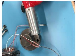
Figure 6: Shrink Butt Splice Connections
