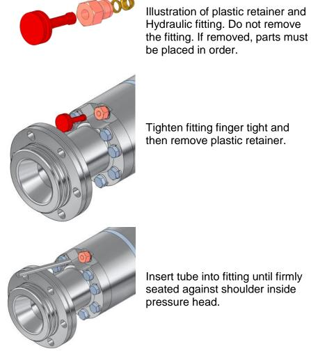
Tighten fitting finger tight and then remove plastic retainer.
