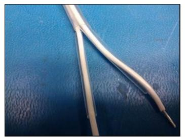
Figure 8: Three Pieces of Shrink Tubing on the Gauge Wires
