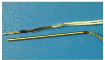
Figure 10: Long Piece of Heat Shrink Tubing Over Both Wires
