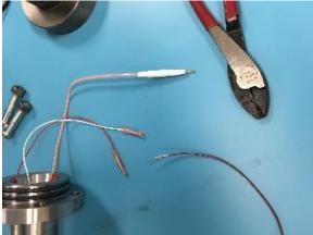
Figure 5: Spy Pro Thermocouple Crimp Connections
