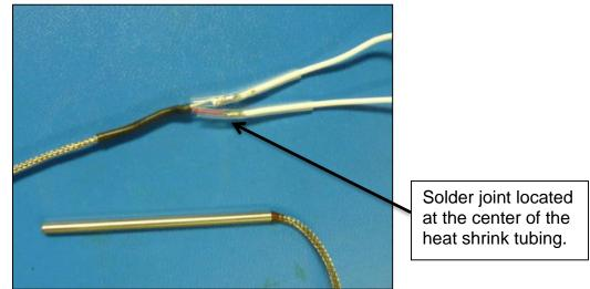
Figure 9: Heat Shrink Tubing Over the Solder Joints
