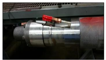
Figure 15: Bench Test Through the Pothead
