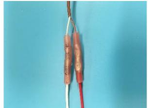
Figure 7: Spy Pro Thermocouple Completed Connections
