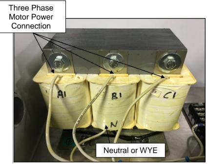
Figure 20: Surface Choke Part Number #99B990
