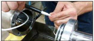
Figure 11: Connect the Motor I-Wire to the Gauge
