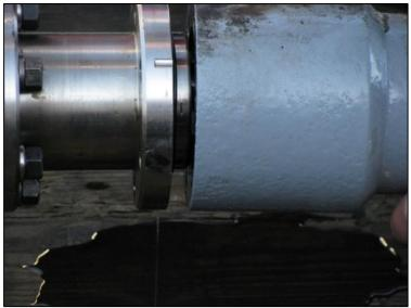
Figure 4: Gauge Stabbed into the Motor Base
