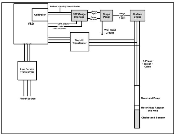
Figure 19: Surface System Wiring Diagram
