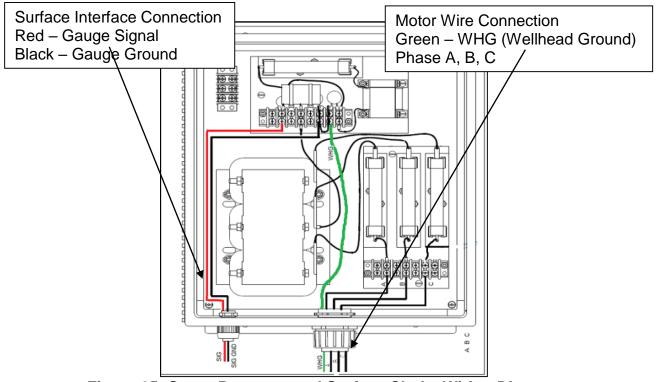
Figure 25: Surge Protector and Surface Choke Wiring Diagram
