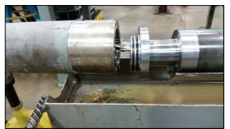
Figure 13: Slide Wire Bundle into the Head of the Gauge
