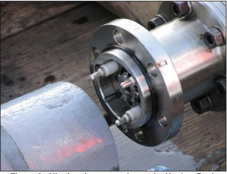
Figure 3: Aligning the motor pins to the Hockey Puck
