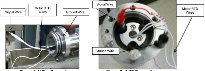
Figure 1: I-Wire Connection
