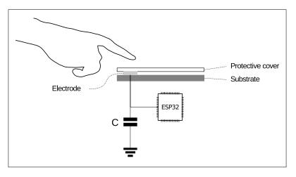
Figure 16: A Typical Touch Sensor Application
