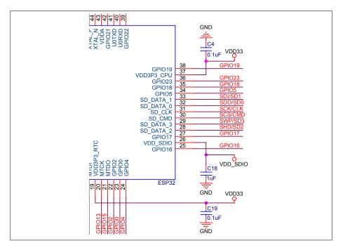
Figure 2: ESP32 Digital Power Supply Pins
