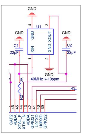
Figure 5: ESP32 Crystal Oscillator
