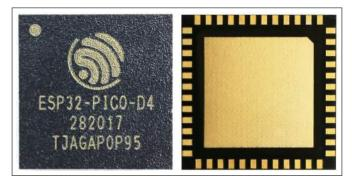
Figure 20: ESP32-PICO-D4 Module
