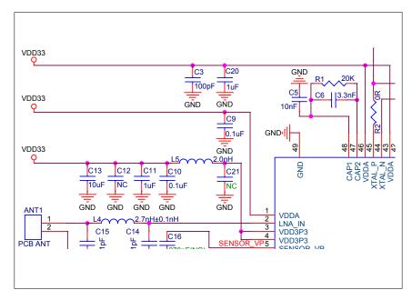
Figure 3: ESP32 Analog Power Supply Pins
