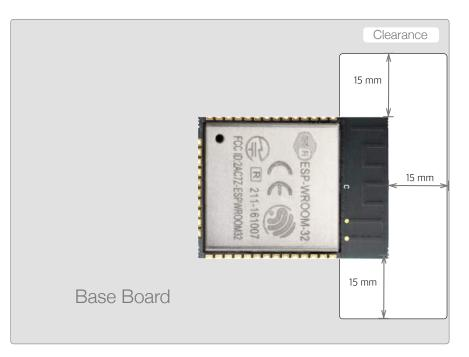
Figure 12: Keepout Zone for ESP32 Module's Antenna on the Base Board
