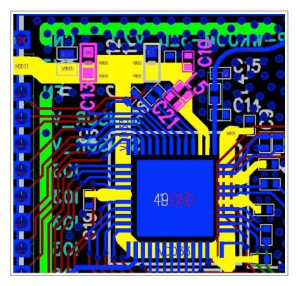
Figure 13: ESP32 Power Supply Design
