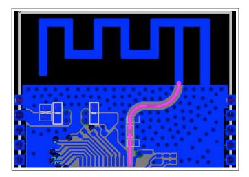
Figure 15: ESP32 RF Layout
