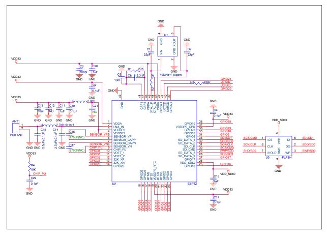
Figure 1: ESP32 Schematics
