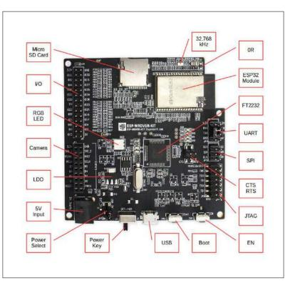
Figure 26: Front Side of the ESP-WROVER-KIT Layout
