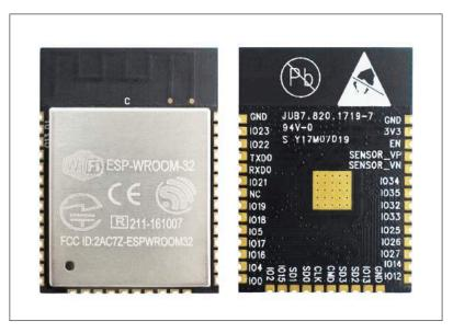
Figure 21: ESP32-WROOM-32(ESP-WROOM-32) Module
