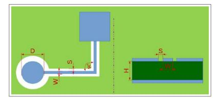
Figure 18: Sensor Track Routing Requirements
