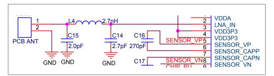
Figure 7: ESP32 RF Matching Schematics
