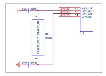
ESP32 supports an external 32.768 kHz crystal oscillator to act as the RTC sleep clock.
