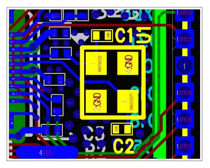
Figure 14: ESP32 Crystal Oscillator Layout
