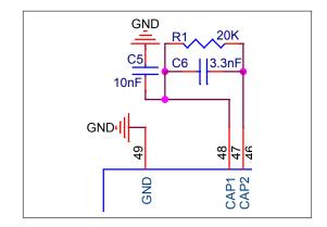
Figure 8: ESP32 External Capacitor
