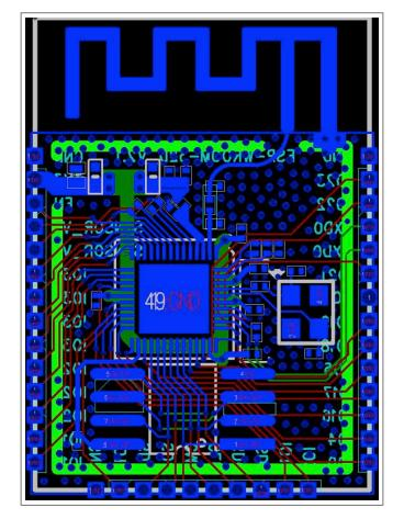
Figure 10: ESP32 PCB Layout
