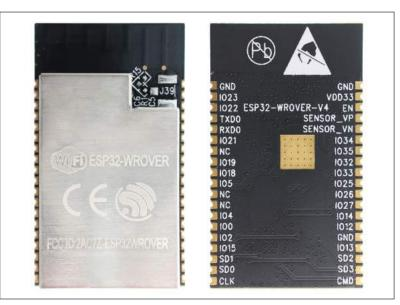
Figure 24: ESP32-WROVER Module
