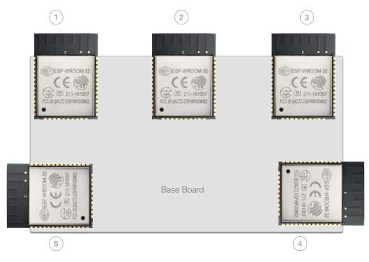
Figure 11: ESP32 Module Antenna Position on Base Board
