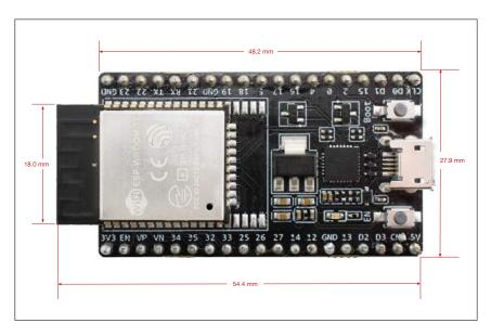
Figure 25: Front Side of ESP32-DevKitC
