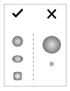
Figure 17: Electrode Pattern Requirements
