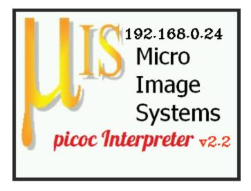
This display is a harmless advertisement for Micro Image Systems and the book *Building Blocks for IOT with your PC and WiFi Peripherals.* It also shows that the ESP32 is running in station mode with an IO address to 192.168.0.24 – your IP address will likely be different. If the ESP32 is running in AP mode it will show the display shown in the following figure.
