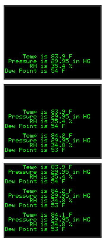
The /oledDemo.c program on the ESP32 provides a simple example of using a 128x64 pixel OLED I2C attached display with the interpreter. To use the o\* functions, OLED must be defined when compiling the ESP32Program sketch. The program's setup function runs the following lines
