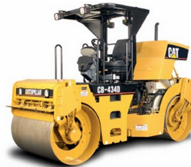
Figure 6. Smooth Wheeled Roller (CAT, 2011).
