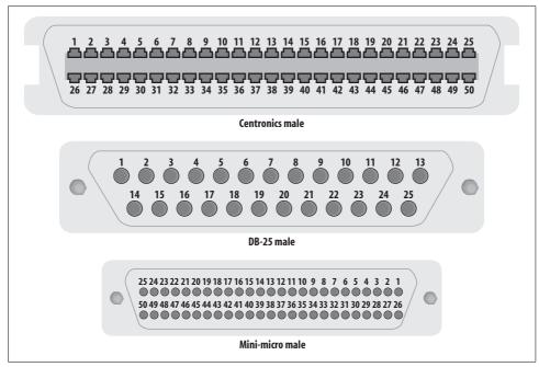
Figure 10-5. SCSI connector pinouts
