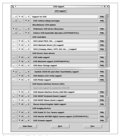
Figure 12-6. Linux USB-related kernel parameters
