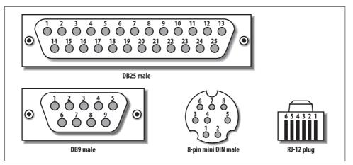
Figure 12-3. Serial cable pin assignments
