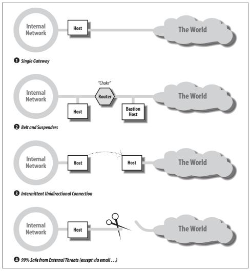
Figure 7-3. Some firewall configuration options
