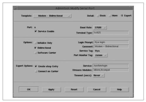
Figure 12-4. Configuring a serial line with admintool
