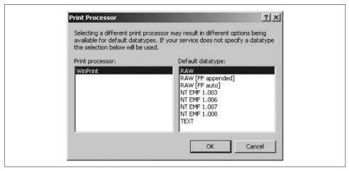
Figure 13-9. Forcing a printer into raw mode operation
