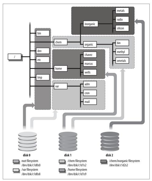
Figure 10-1. Mounting disk partitions within the Unix filesystem
