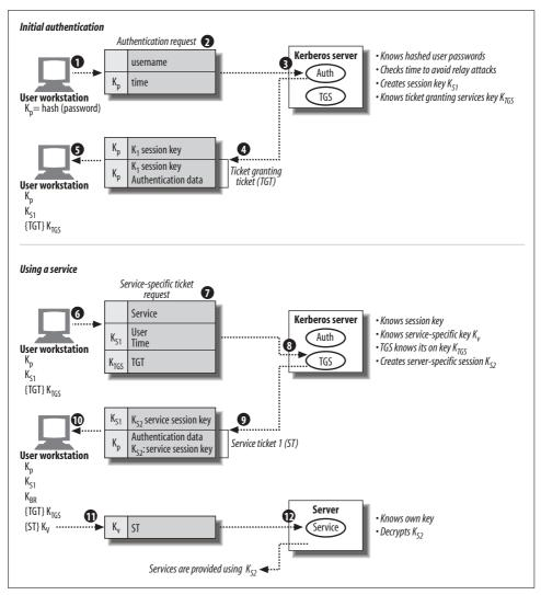
Figure 7-1. Basic Kerberos 5 authentication
