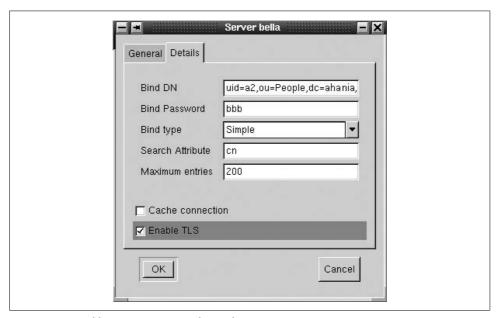
Figure 6-14. Enabling TLS support in the gq client
