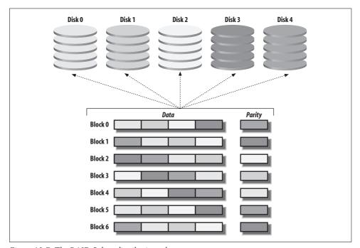
Figure 10-7. The RAID 5 data distribution scheme
