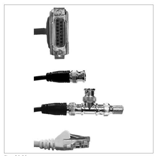
Figure 5-2. Ethernet connectors
