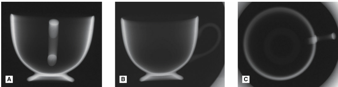
FIG. 1.11 Three two-dimensional radiographs of the same teacup illustrated in Fig. 1.10. (A) The front view shows only the outline of the teacup and the shadow of the handle, but gives no information as to which side of the cup the handle is located or its shape. (B) The side view again shows the outline of the cup and also the shape of the handle. (C) The plan view confirms the teacup is round and shows the position of the handle, but provides no information on the height of the teacup or the shape of its base.
