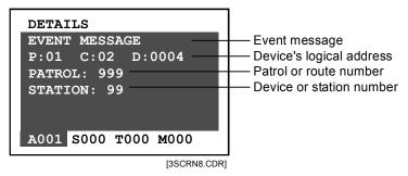
The Details panel shows the event or state of the off-normal station, as well as the logical address, patrol or route number, and station number of the device.
