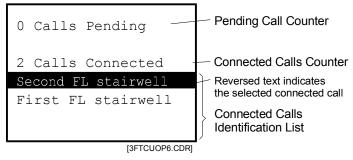
Figure 4-6: 3-FTCU Display, Two Connected Calls
