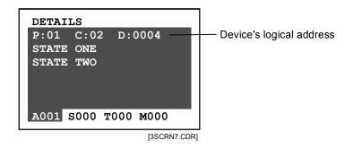
If a device activation causes the event, pressing Details displays the active device's logical address in the following format:
