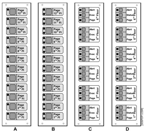
Figure 3-2: Control/display module options
