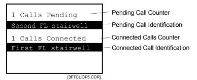
Figure 4-5: 3-FTCU Display - One Connected Call and One Pending Call
