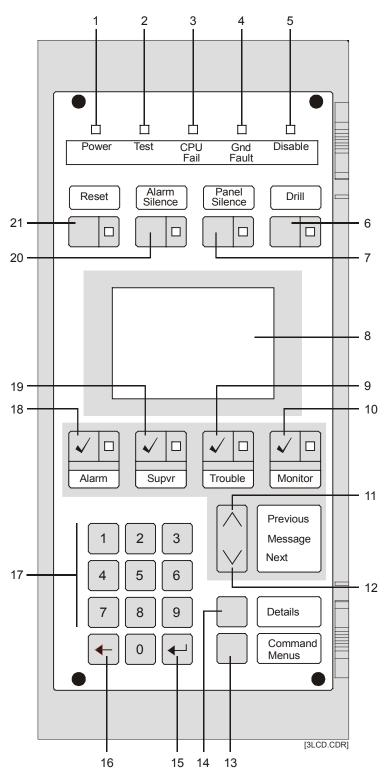
Figure 2-1: 3-LCD controls and indicators
