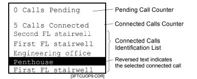
Figure 4-7: 3-FTCU Display, Five Connected Calls
