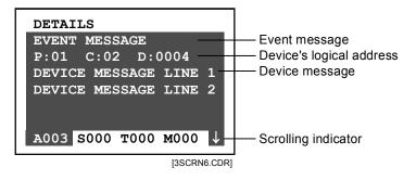
Each device panel shows the event message or state of the device, the device address, and the device message (usually the device location) which can be one or two lines long.
