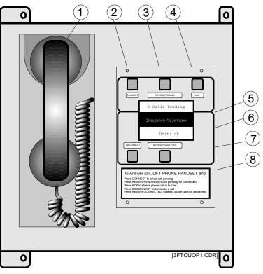
Figure 4-1: 3-FTCU controls and indicators
