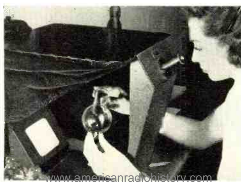
Polariscope is here used to inspect glass bulbs for flaws or strain which may occur during the shaping operations
