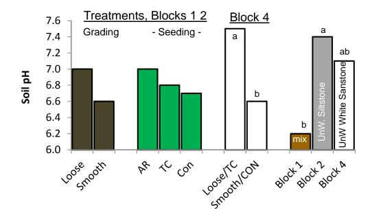
**Figure 1.** Soil pH on reclamation areas (treatment plot means). Different lowercase letters within groupings indicate statistically significant differences.
