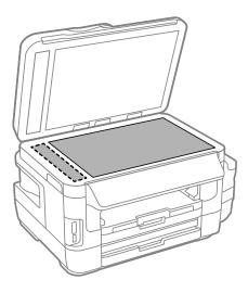
**Note:** If lines appear on the printout or in scanned images, carefully clean the scanner glass on the left.
