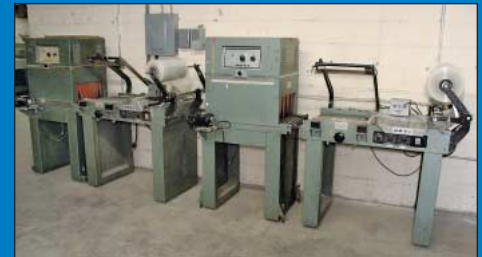
(2) Weldtron Heat Shrink and L-Seal Packaging Lines
