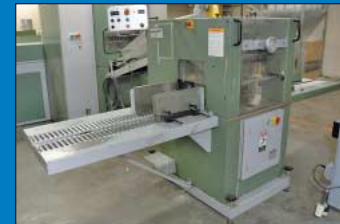
Muller Martini Model 3006 "Star Bind" Perfect Binding Line - Model Uno Type 1534 Stacker View
