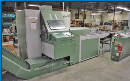
Muller Martini Model 3006 "Star Bind" Perfect Binding Line - Merit "S" Type 3671 Three-Knife Trimmer View
