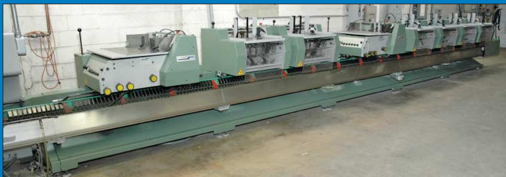
1997 Muller "Bravo" Six-Pocket Saddle Stitcher - Pocket and Cover Feeder View
