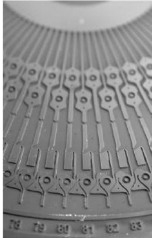
Microfluidic mold etched in Si by DRIE
