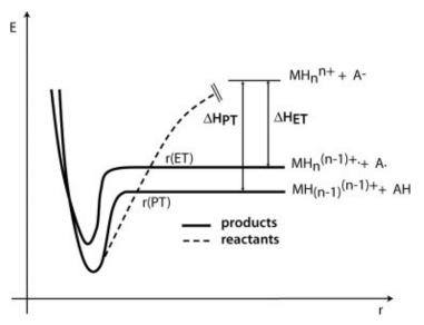
Fig. 3. Schematic potential energy curve of an ion/ion reaction between a peptide precursor [MHn]n1 and a reagent anion A2. As the entrance channel crosses the exit channels of either electron or PT, the reaction can occur. With regard to ET happening at greater distances, this reaction is more likely than PT for the typical anion/cation pairs. Slightly modified after [26].
