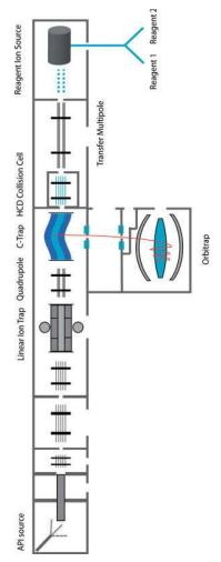
Fig. 4. Scheme of the newly developed LTQ-Orbitrap XL with ETD. The reagent ion source is implemented at the back side of the instrument. Slightly modified after [22].
