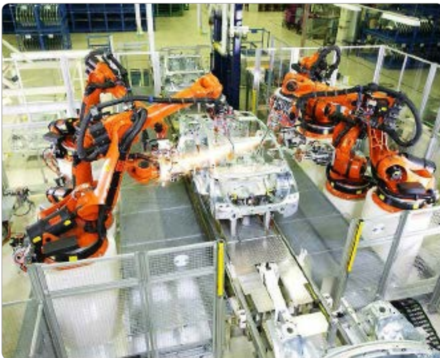
Robotic cell-based solutions for spot welding (Photo: KUKA Systems)
