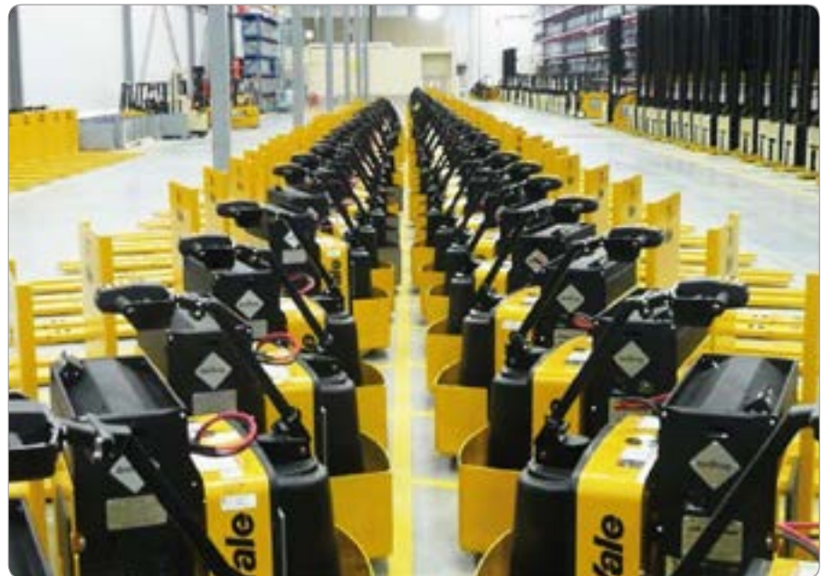
FC systems can easily be retrofitted to replace lead-acid batteries into forklifts, like in these Yale machines
