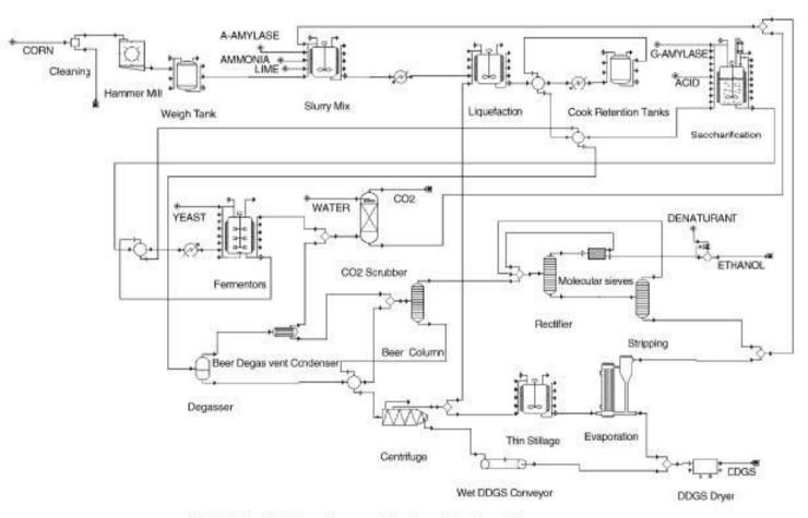
Fig. 1. Simplified flow diagram of the dry-grind ethanol from com process.
