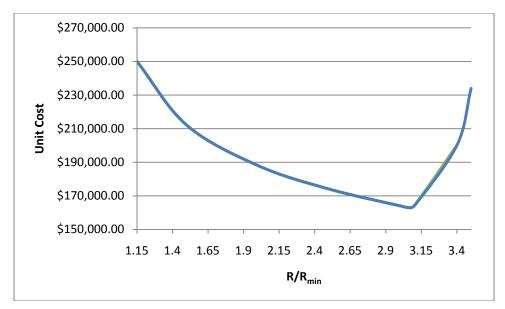
Figure 4.4: Determination of the Optimal Reflux Point for Tower T-102
