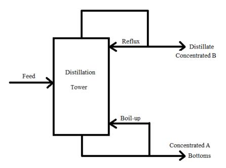
Figure 2.2: Schematic of Traditional Distillation
