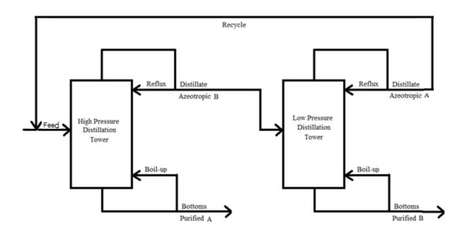
Figure 2.3: Schematic of Pressure-Swing Distillation
