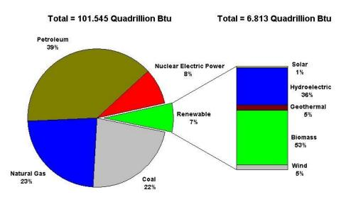
Figure 2.1: Consumption of Energy in United States in 2007 Broken Down by Source
