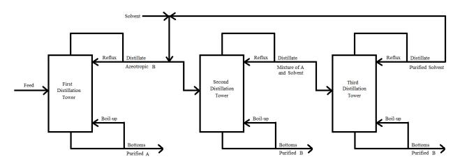
Figure 2.4: Schematic of Extractive Distillation
