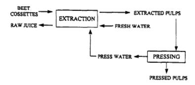
Figure 3.1: Outline of Sugar Extraction and Press Water Production in a Sugar Beet Factory (Bogliolo et al., 1996)
