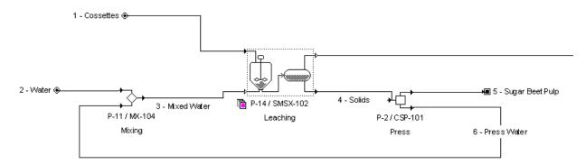
Figure 4.1: The Sucrose Extraction Section Modeled in SuperPro Designer
