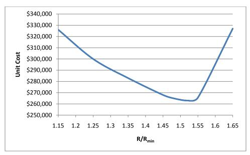
Figure 4.3: Determination of the Optimal Reflux Point for Tower T-101
