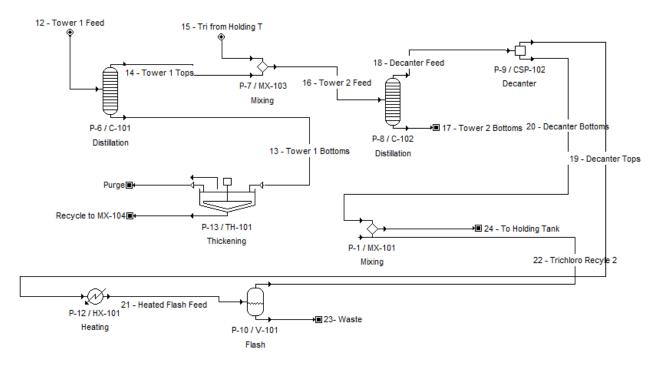
Figure 3.3: Extractive Distillation Process
