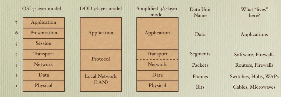
OSI (Open Systems Interconnection) mnemonic: All People Seem To Need Data Processing We'll be using the "simplified model," and talking mostly about the Network (IP) and Transport (TCP and UDP) layers, plus a little about Data (Ethernet details).
