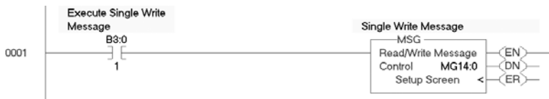
Figure 6.21 Example Ladder Logic Explicit Messaging Program for Write Single
