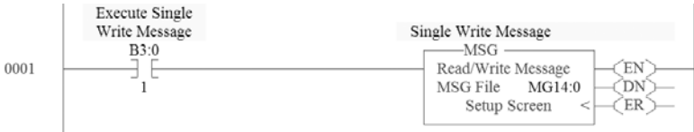
Figure 6.53 Example Ladder Logic Explicit Messaging Program for Write Single
