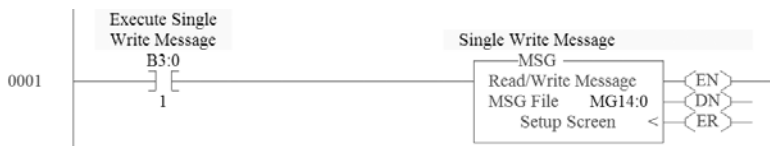
Figure 6.47 Example Ladder Logic Explicit Messaging Program for Write Single
