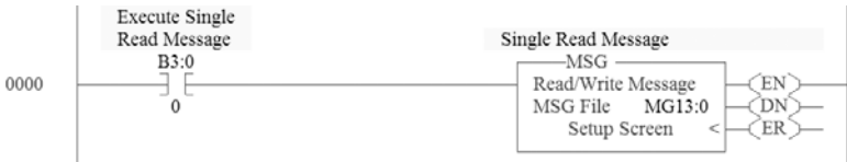
Figure 6.50 Example Ladder Logic Explicit Messaging Program for Read Single
