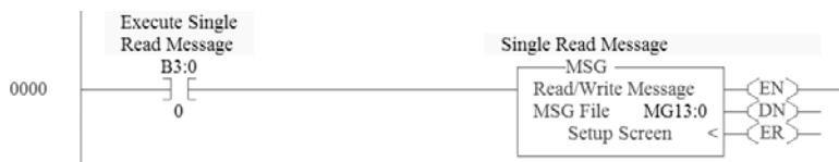
Figure 6.44 Example Ladder Logic Explicit Messaging Program for Read Single
