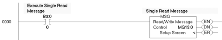
Figure 6.18 Example Ladder Logic Explicit Messaging Program for Read Single
