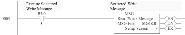
Figure 6.60 Example Ladder Logic Explicit Messaging Program for Write Multiple
