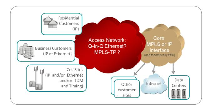
The core is richly connected, while access network topologies are typically tree or ring configurations. Thus a fault in the access network affects fewer people than a fault in the core, but there are fewer bypass options. The core can get away with fast re-route (FRR) while the access network requires OAM and planned Automatic Protection Switching (APS).
