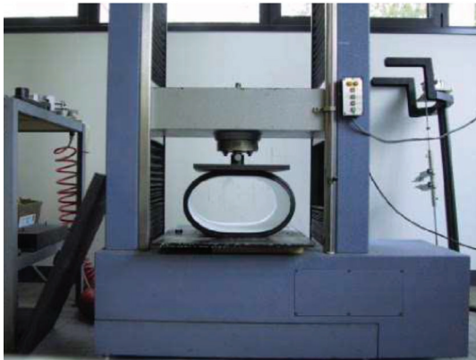
Figure 4.1: Test piece of corrugated pipe DN 315 with 30% deflection of outside diameter
