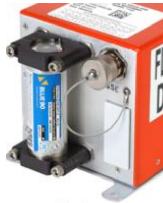
90 days ULB attached to recorder (37,5Khz - 2,5NM)
